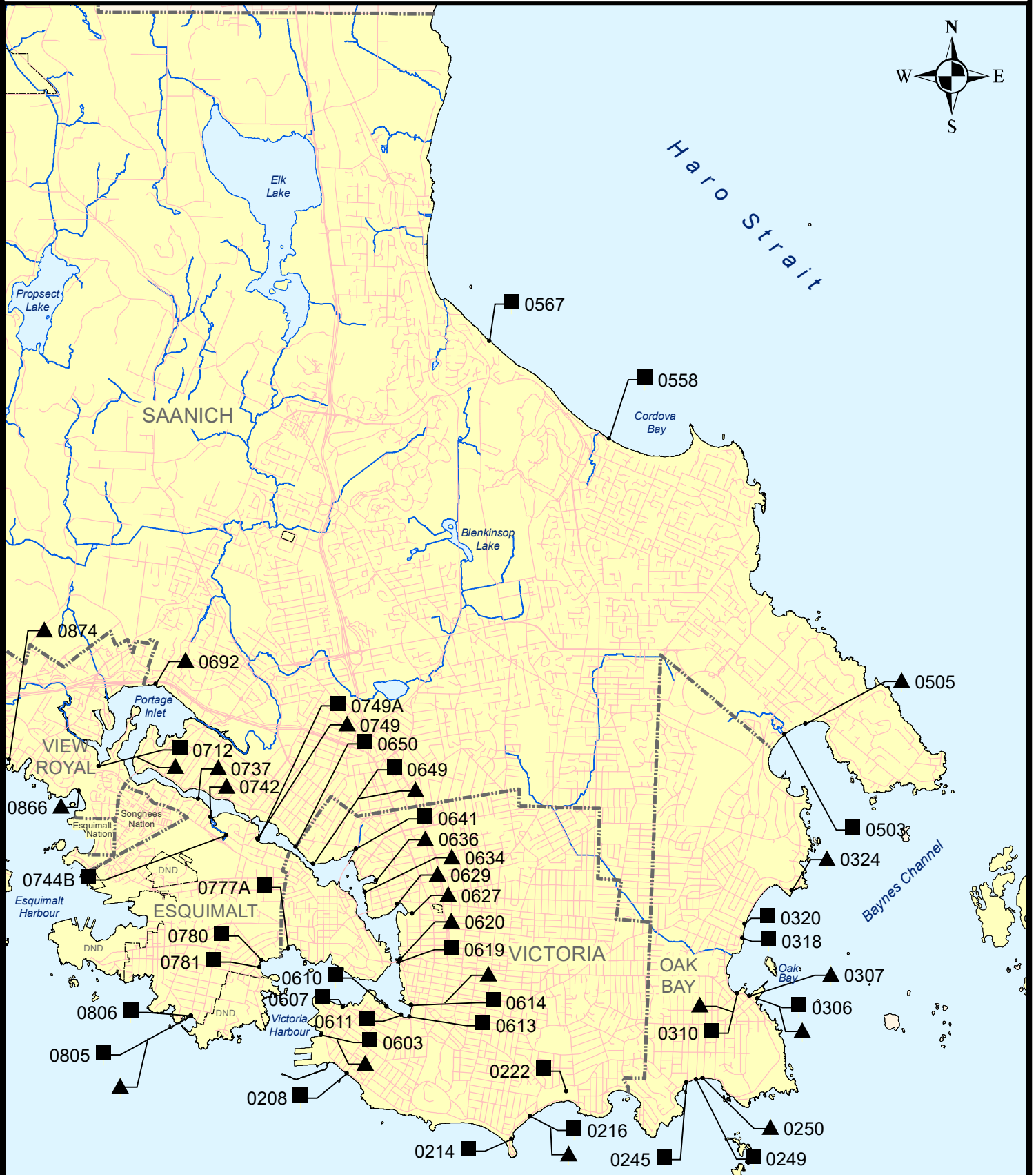
Figure C - Core Area 2019 Stormwater Discharges Requiring Action for Public Health and Environmental Concerns (Esquimalt to Central Saanich Border)
