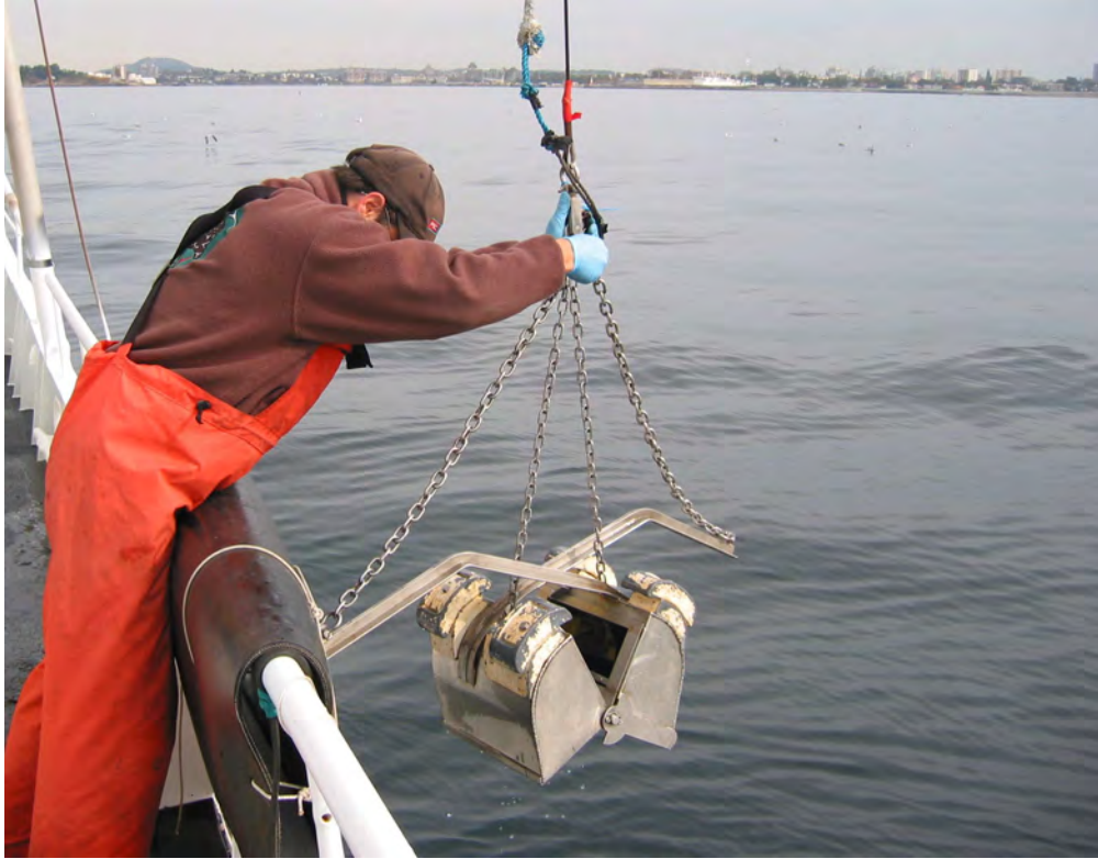
Picture 4.1 Seafloor Sampling Van Veen Grab
