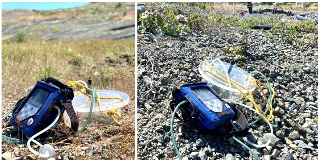
Photo 4.10a & 4.8b - Flux Chamber Measurement at Hartland Landfill
