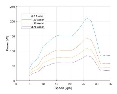
Figure 5: Human power contributions for various assist levels with impacts of grade removed. Filtered to only include power corresponding to grades less than 2%.
