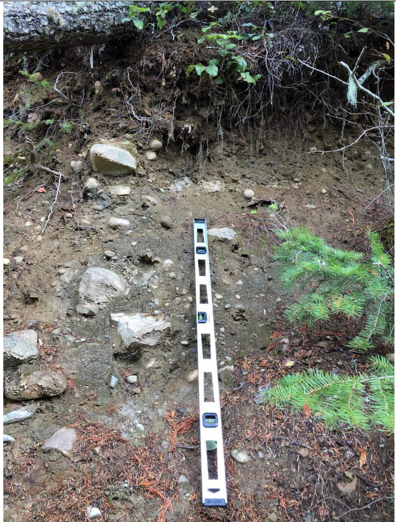
Photo 07: Sloughing/slope erosion observed just above the eastern waterline of the reservoir (Photo 1 of 2).
