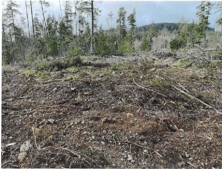
Photo 9 – Native dense brown silty gravelly soil exposed at the Proposed Building Site on Lot 9.
