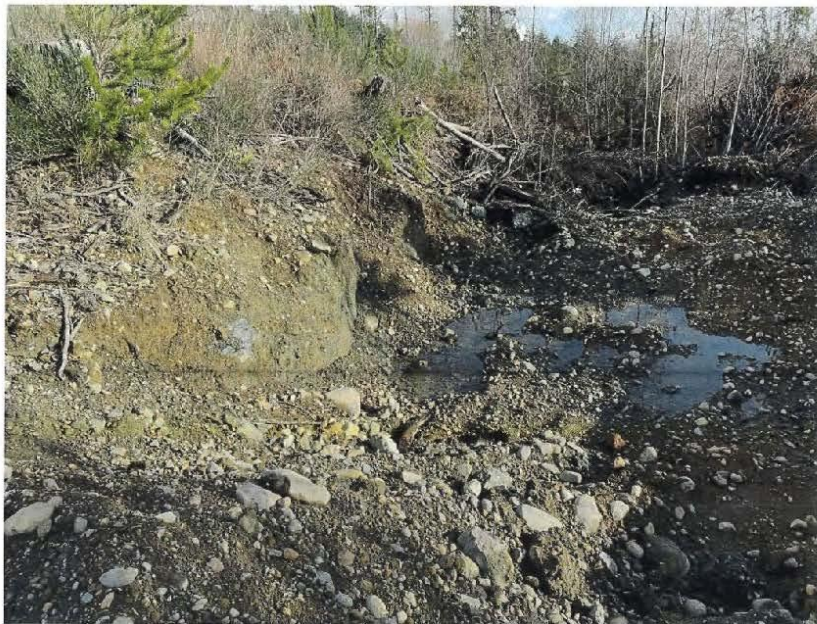
Photo 21 – Typical soil exposure on site of brown very dense gravelly silt (till)
