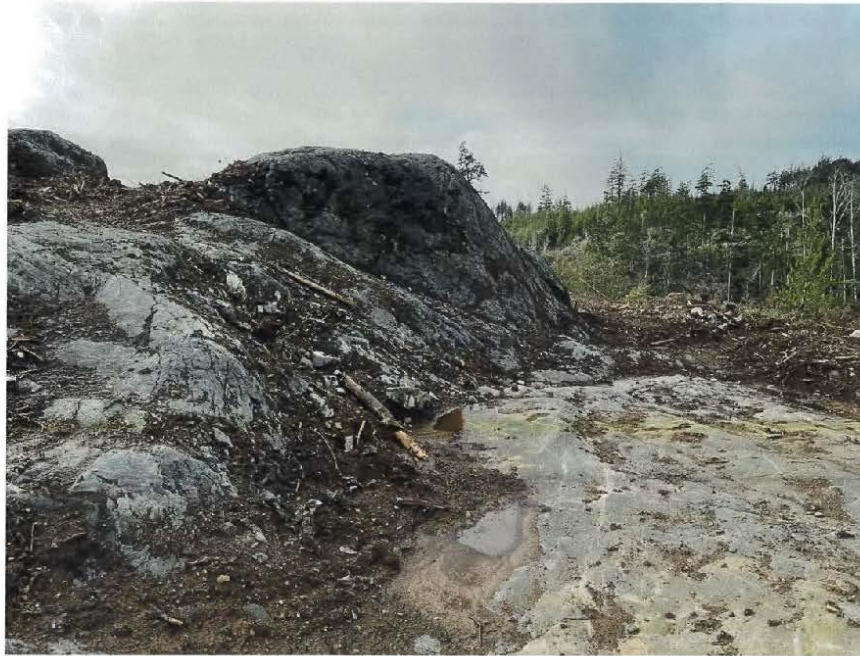
Photo 17 – Typical rounded weathering profile of bedrock exposed on Lots 15, 16 and 17
