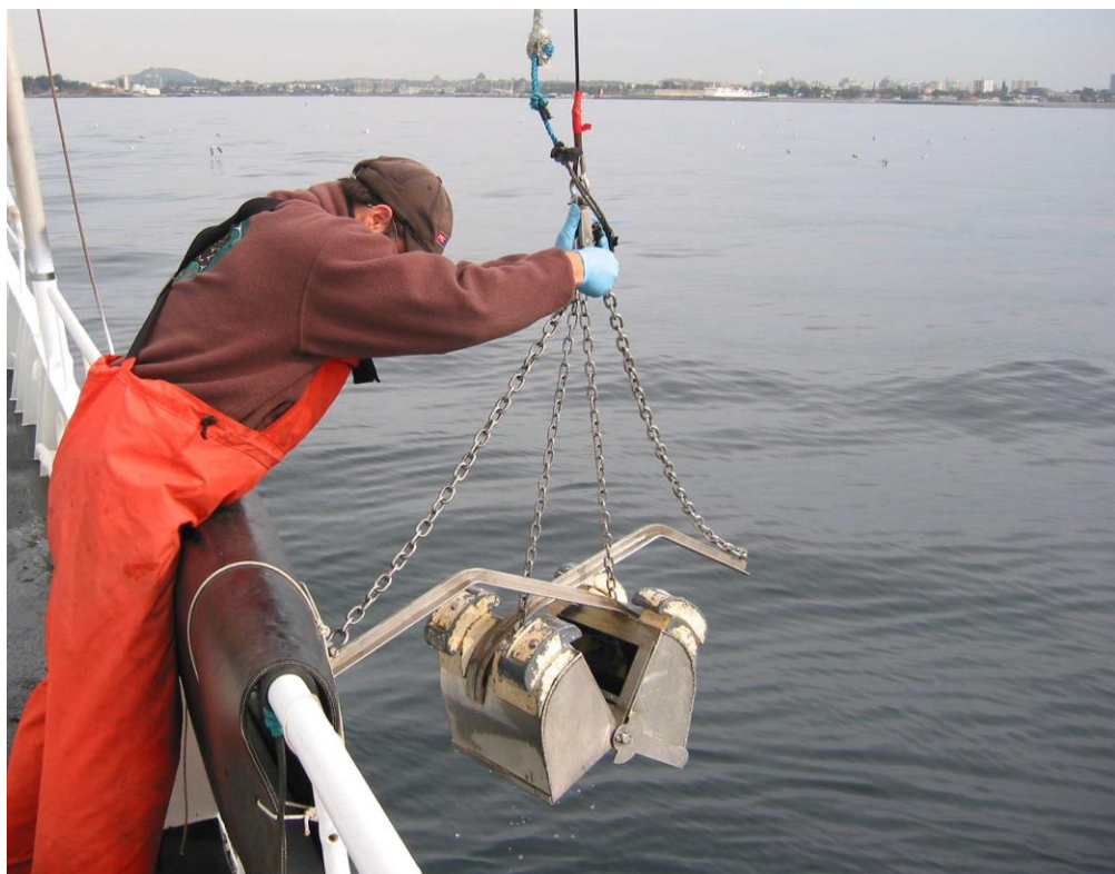
Picture 5.1 Seafloor Sampling Van Veen Grab
