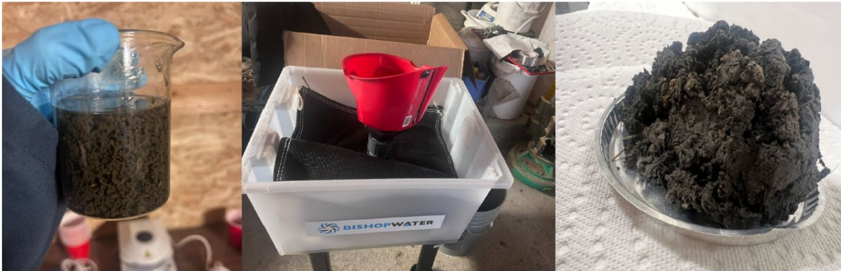
Onsite jar testing (left), Geotube® Dewatering Test (GDT) (middle) and GDT After 2 months - 21% (right).
