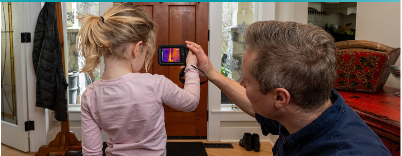
Family looks at their home through a thermal camera to detect insulation gaps.
