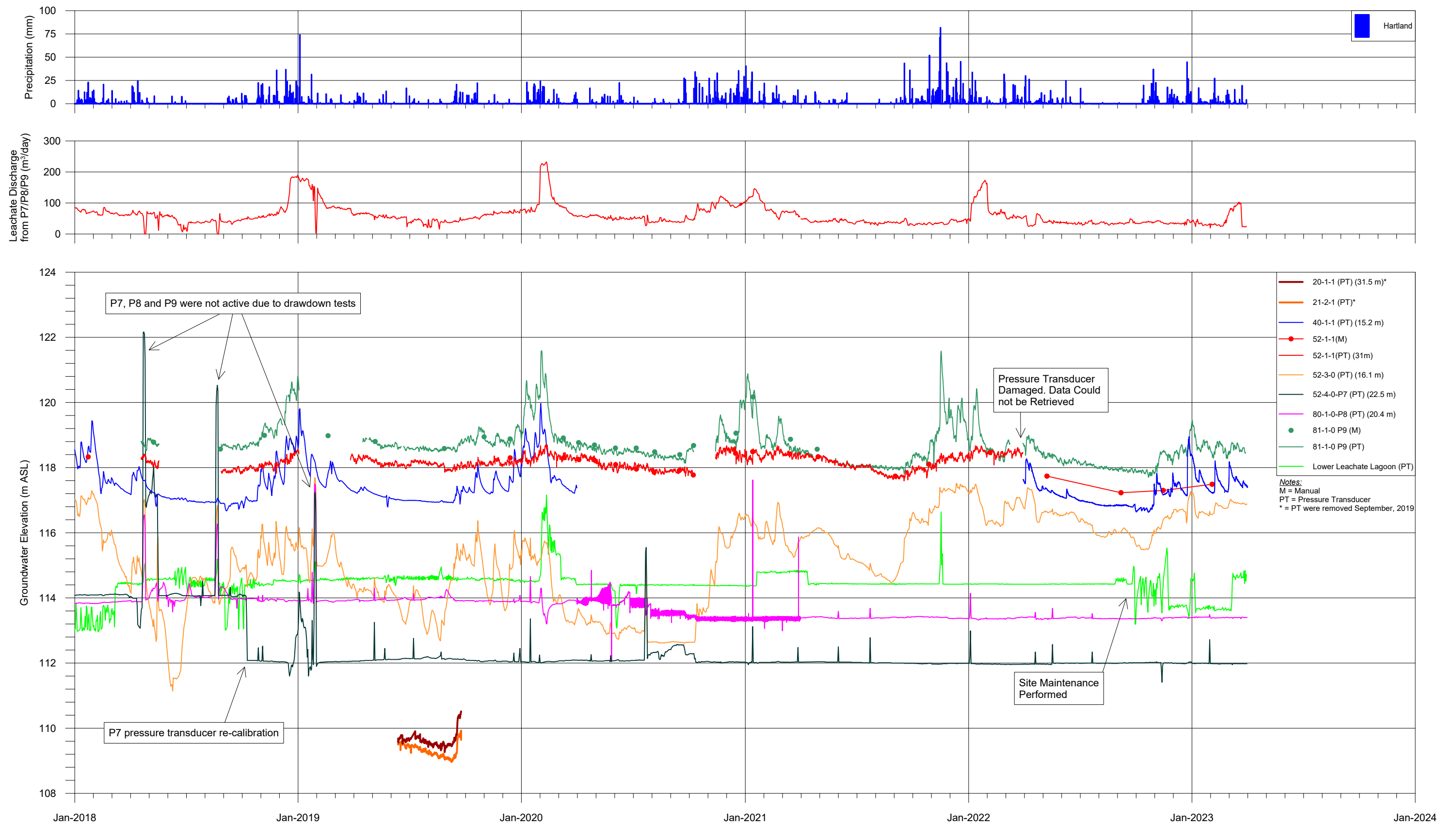
Figure 4-6. Groundwater Elevations Surrounding the North Purge Wells
