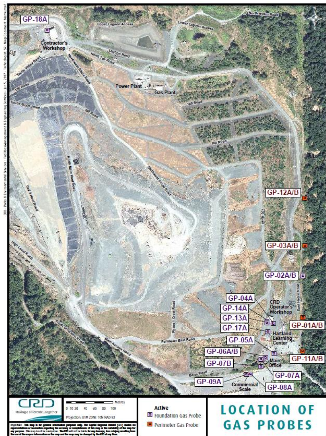
Figure 8 Location of Gas Probes
