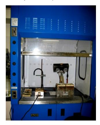
Note: The *Occupational Health and Safety Regulation* states a fume hood must not be used for storage of chemicals <u>unless</u> it is used exclusively for this purpose and is labeled with this limitation.
