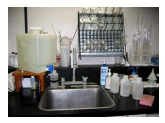
Sinks and drains in the laboratory are prime locations for wastes to enter the sewer. Following the best management practices and minor plumbing modifications listed below will help reduce the likelihood of spilled chemicals or waste entering the sewer through your sinks or drains. See Metals for information on sediments that may be contaminated (with mercury, for example) accumulating in sink drainpipes on page 15.
