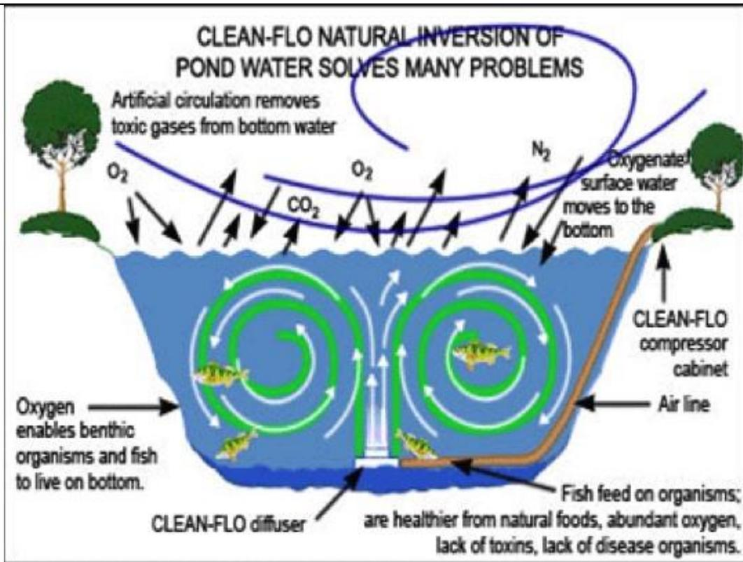
Figure 9.3 Clean-Flo laminar flow aeration system
