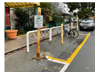
Example of ‘Coat Hanger’ rack type which does not meet best practices
