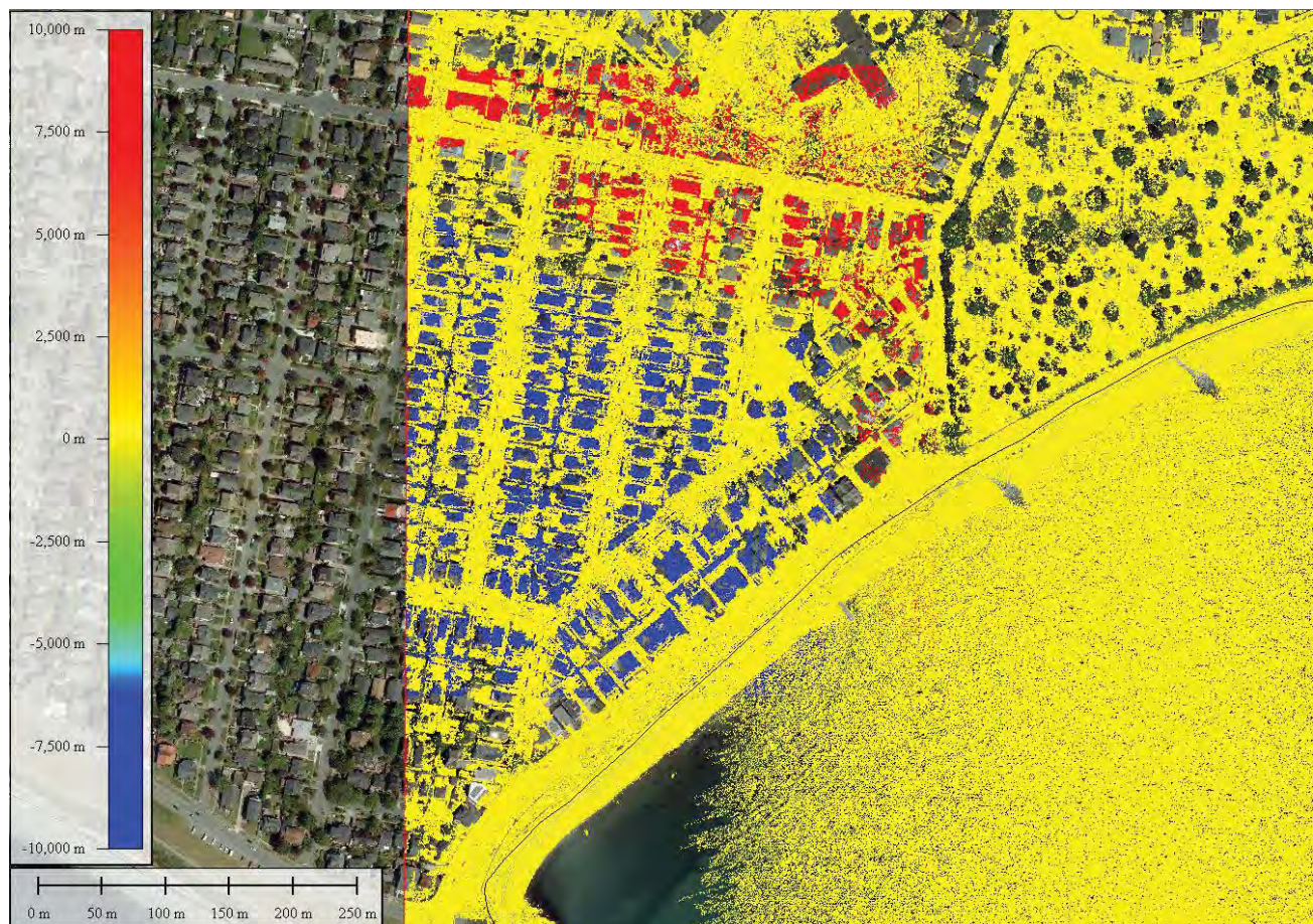
Figure 3-4 LiDAR Point Cloud Artefacts
