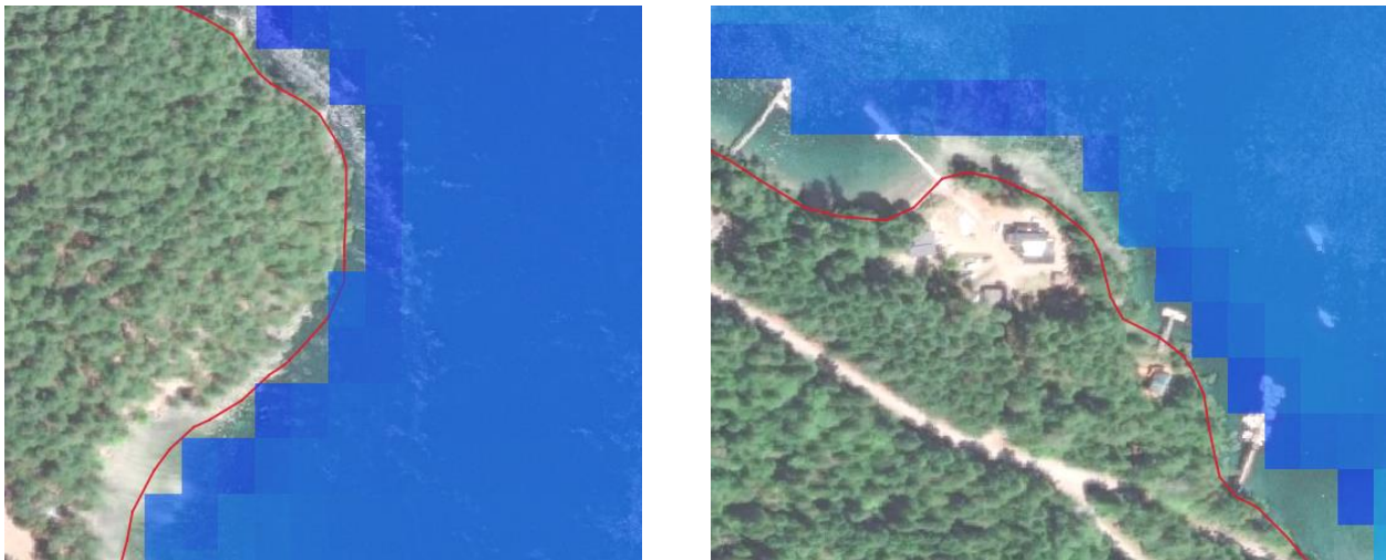
Figure 4-26 Examples of Coarse Grid Results Not Inundating the Coastline Boundary Due to Model Resolution
