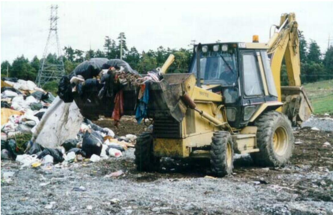
**Photo 2-1. Backhoe with Three Way Front Bucket Loading Sample**
