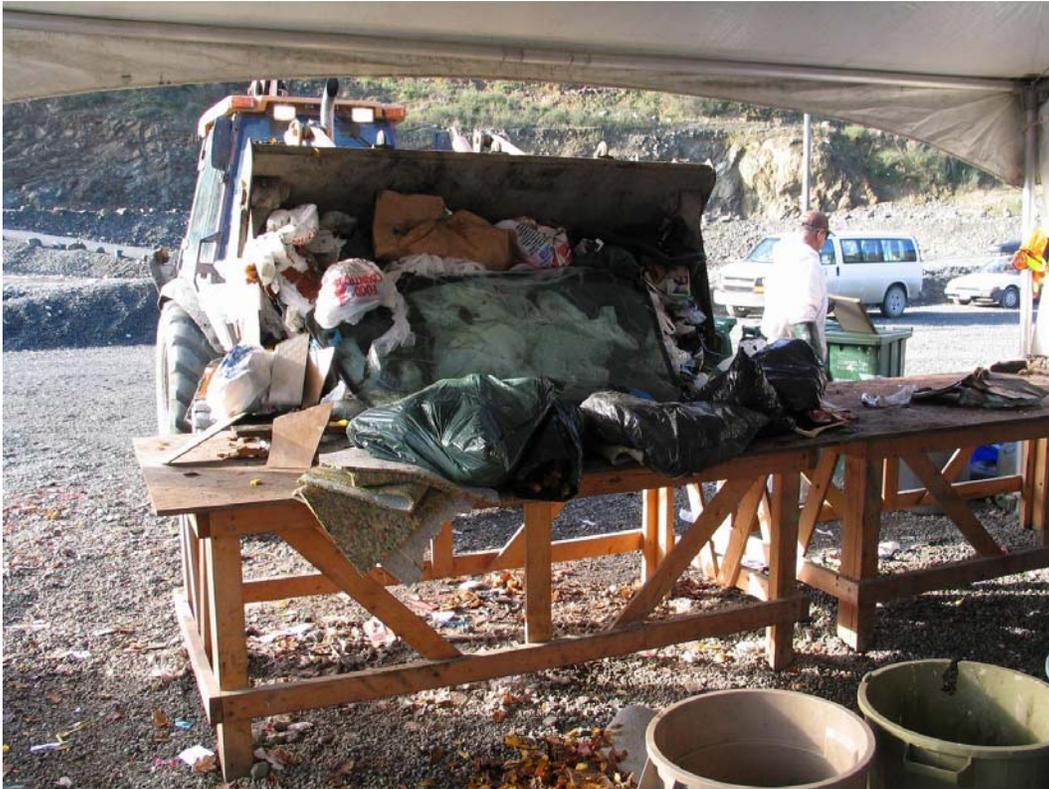
**Photo 2-2. Loader with Three-Way Front Bucket Unloading a Sample.**
